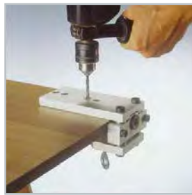
Drill the adjustment hole. Max opening of 1-3/4"
